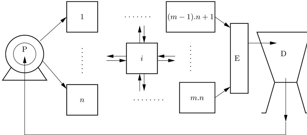
Figure 7: Scheme of spatial discretisation of a photobioreactor with recycle.
