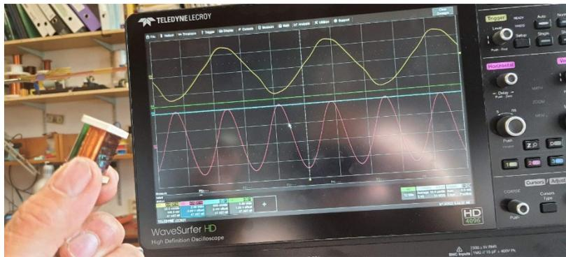
Fig. 5 - 50  $\mu$ T field for tuned excitation
