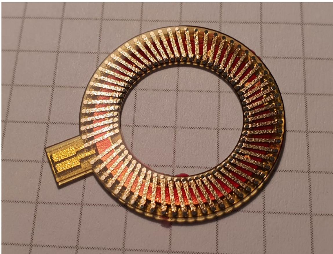
Fig. 1 - Photo of the final printed sensor
