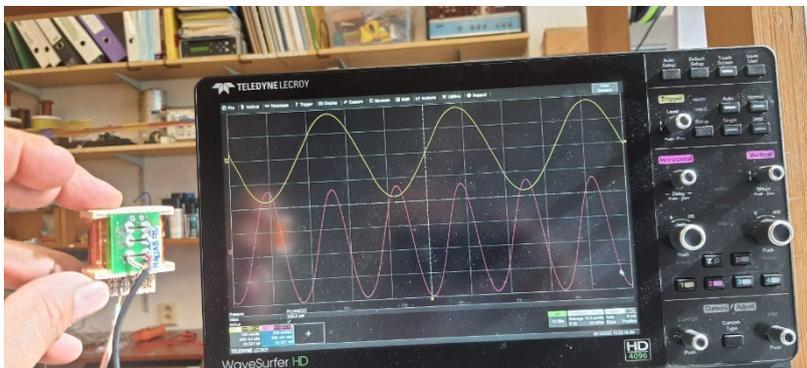
Fig. 4 - 50  $\mu$ T field - thanks to the resonance tuning the response is quite clean 2<sup>nd</sup> harmonic voltage
