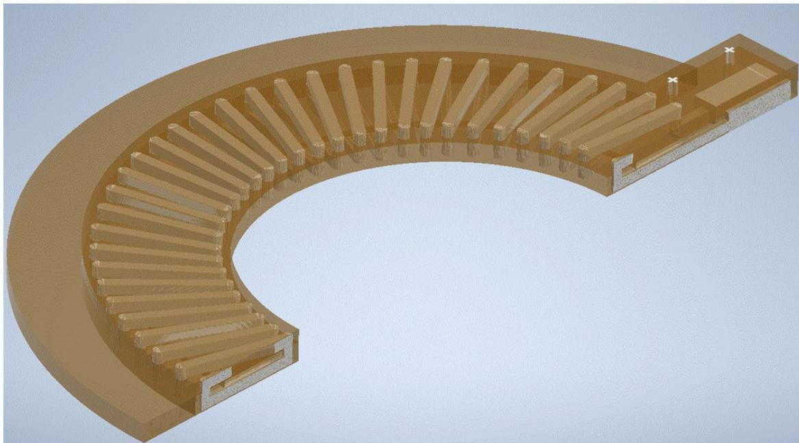
Fig. 2 - Fluxgate sensor model crossection
