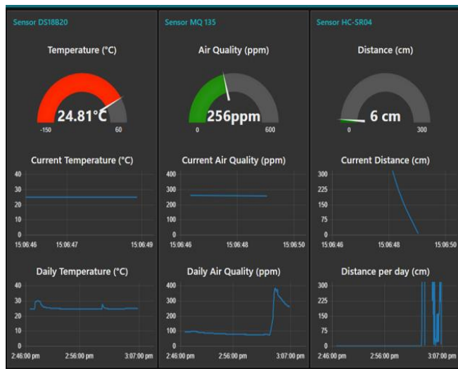
Fig. 12. The Graphical User Interface: the value measured by the smart jacket.
